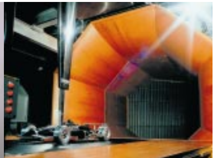
DESIGNED BY STUDENTS, THE COMPETITION WINNING REYNARD RACE CAR IS TESTED IN AN OPEN JET WIND TUNNEL
